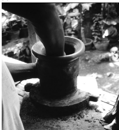
PHOTO 13.11a An (exceptionally male) potter in San Carlos City, Negros Oriental, Philippines shapes a vessel on a turntable by opening a lump of clay, then shaping the rim and continuing by thinning the rest of the lump somewhat between his hands.
