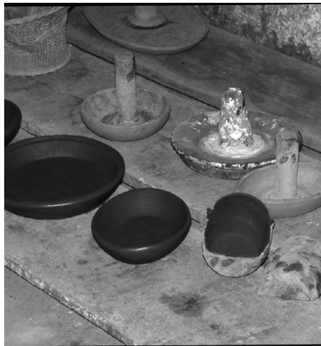
PHOTO 13.14 In Michoacán, Mexico, open vessels (bowls, plates, etc.) are shaped horizontally by placing a pancake of clay over a mushroom-shaped mold made by attaching a handle to an upside-down, fired, bowl. The potter shapes the vessel by hand against the mold, then shapes the rim by removing excess clay with a wire held between the teeth and one hand while rotating the mold. The photo shows two molds for open vessels above the resultant vessels, and one closed vessel in a vertical half-mold.
